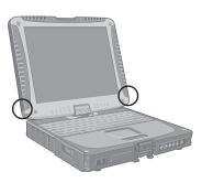
The tether can be attached to the bottom right or bottom left corner of the display. It prevents the stylus (included) from falling accidentally.
