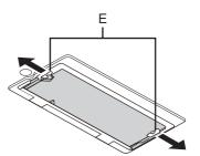
2 Carefully remove the RAM module from the slot.
