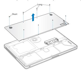
*Important:* When you remove the bottom case, you expose sensitive internal components. Avoid touching anything other than the memory assembly when you remove and replace memory.
