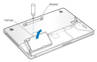
The bracket detaches from the drive. Put it aside in a safe place.
