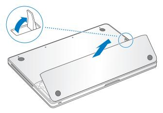
*Note:* The latch must be in its released, open position to remove and replace the battery and access door.
