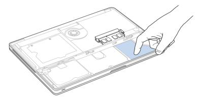
4 Push the ejection levers on the sides of the memory module in an outward direction to release the module from the memory card slot.
