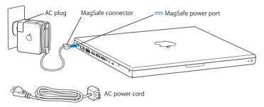
To extend the reach of your power adapter, first pull the AC plug up to remove it from the adapter. Attach the included AC power cord to the adapter, making sure it is seated firmly. Plug the other end into a power outlet. The AC power cord provides a grounded connection.
