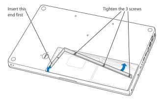
5 Replace the L-bracket by inserting the short end first and tightening the screws.
