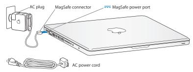
To extend the reach of your power adapter, replace the AC plug with the AC power cord. First pull the AC plug up to remove it from the adapter, and then attach the included AC power cord to the adapter, making sure it is seated firmly.
