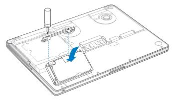
9 Replace the bracket and tighten the screws.
