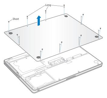
*Important:* When you remove the bottom case, you expose sensitive internal components. Avoid touching anything other than the hard drive assembly when you remove or add a hard disk drive.
