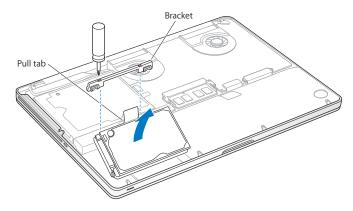
6 Hold the drive by its sides while you gently pull the connector on the left side of the drive to disconnect it.
