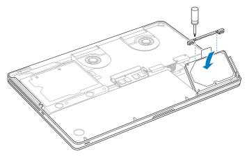
9 Replace the bracket and tighten the screws.
