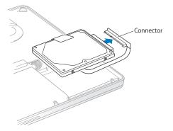
The connector is attached to a cable and remains in the hard disk drive bay.
