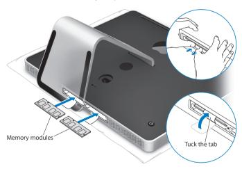
11 Replace the memory access door using a Phillips #2 screwdriver to tighten the screw.
