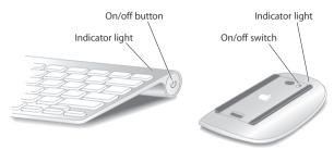
When you first turn on your keyboard or mouse, the indicator light glows steadily for 5 seconds, indicating the batteries are good. Then the indicator light blinks until you turn on your iMac and a connection is established. If your keyboard or mouse don't turn on, make sure batteries are installed properly and charged (see page 47).
