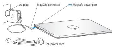
To extend the reach of your power adapter, replace the AC plug with the included AC power cord. First pull the AC plug up to remove it from the adapter, and then attach the AC power cord to the adapter, making sure it's seated firmly. Plug the other end into a power outlet.
