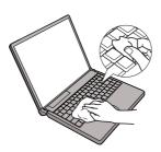
Slowly lift up the computer, keeping it level, and wipe any water coming out of the holes on the bottom using a soft, dry cloth.
