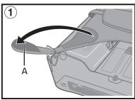
① Remove the edge (A) of hand strap passing through the clip. (The illustration shows the left side of hand strap as an example.)
